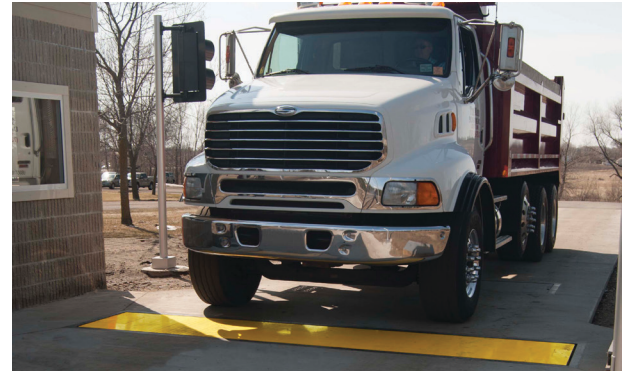
The LS-WIM System provides an effective method to track the volume of bulk materials going in, and leaving, any yard where inventory needs to be tracked.
